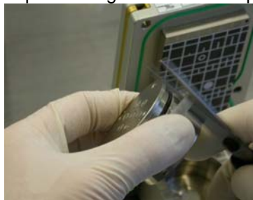
Mounting of locking cover:
