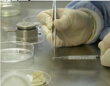
Implementing PP-felt in bottom of PCC:
