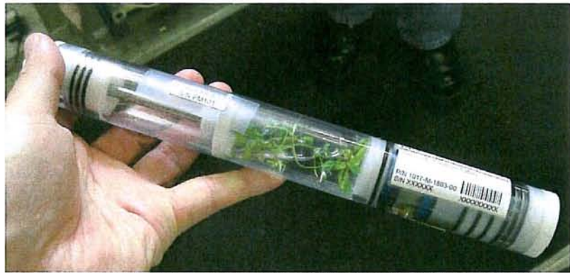
Figure 2. Kennedy Fixation Tubes showing how the plant samples will be contained in fixation liquids. The KFTs have sets of 3 o-rings to contain the samples.
